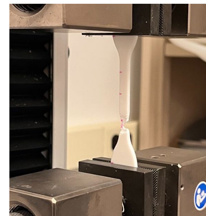
Figure 3: Tensile Test of PLA Printed at 0°/90° raster angle on Instron 3345 Universal Testing System. Gauge length and clamp positions according to D638
